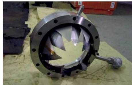
Open rupture disc
