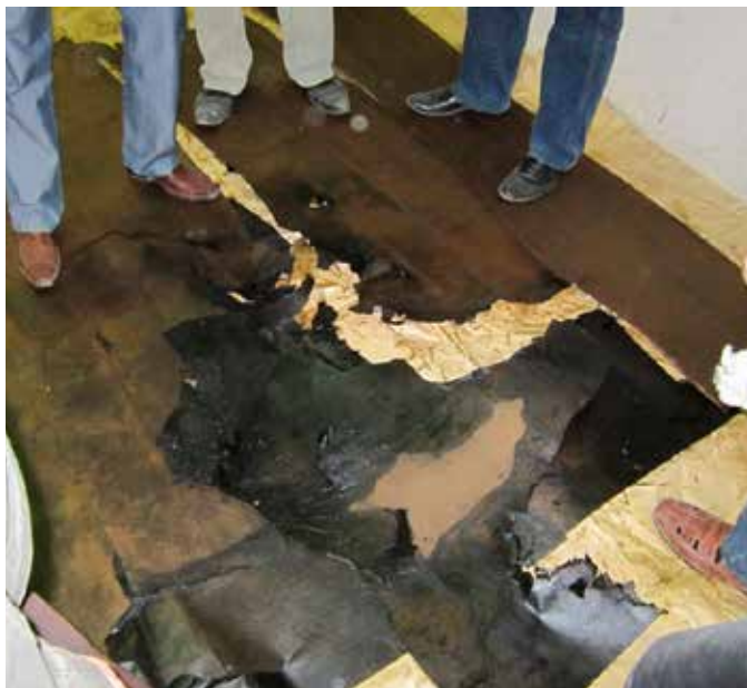
Figure 2: Burnt cardboard insulation
