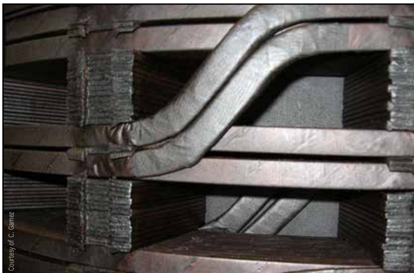
Figure 6: Example of transformer turns with degraded paper
