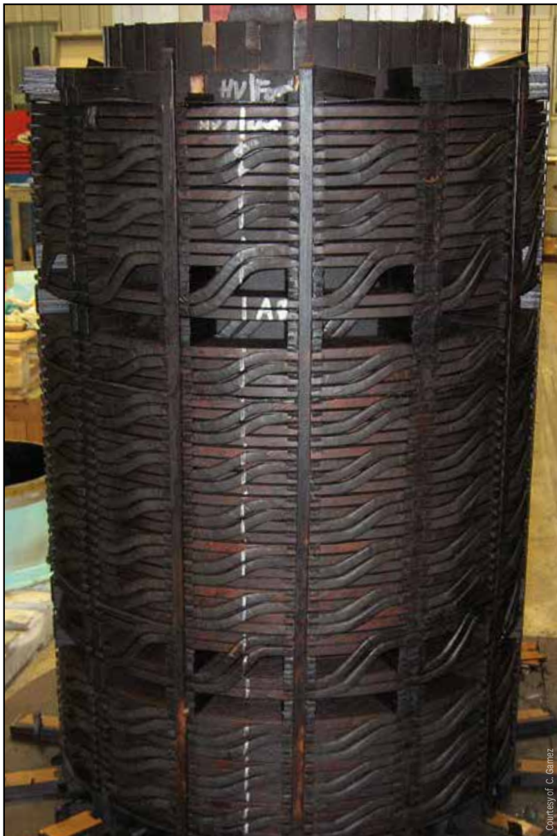
Figure 5: Example of transformer coil with degraded paper
